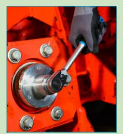
Operating using ratchet with inserted ½" (12.5 mm) 4-point socket
