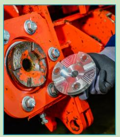
Tool with suitable profile for quick coupler
